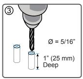
Drill 1" (25 mm) depth hole with 5/16" drill bit.
