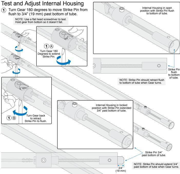
2 To make adjustments, remove the Gear and move the Fixed Rack. Insert the Gear and repeat Step 1 above to test again. When Internal Housing is properly set, proceed with next step.
