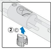
NOTE: For small adjustments, turn Strike Pin clockwise or counter clockwise into Connecting Stud.
