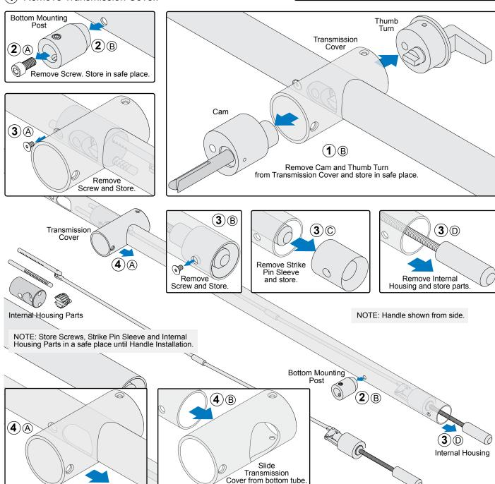
DISASSEMBLE EXTERIOR HANDLE
