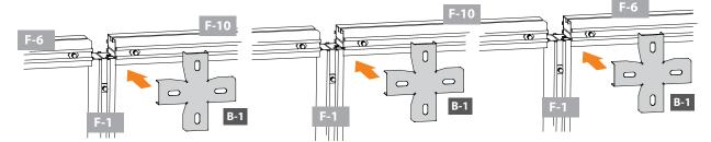
3.5B Secure each B-1 connector with three bolts.
