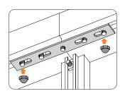
2.7C Loosen set screws on side profiles and slide down. Fit wide part of B-3 connector onto set screw, slide up into place fitting gutter set screw at other end. Tighten set screws and secure with bolts.
