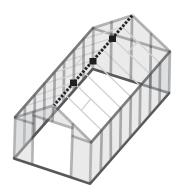
7.1 Prepare the two R-1 and two R-1E roof profiles. They will line up in a row and joined using three B-5 connectors using a total of fourteen set screws and three long hex bolts. Arrange profile so bolt track is facing up.
