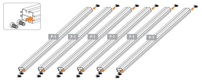
8.10 Measure 195/e inches from one side of profile. Slide middle set screw to that point and tighten to hold in place. Tighten the other two set screws on each end of profile.
