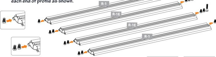
7.1B Line up four profiles in a straight line with R-1E profiles in the middle. Hand tighten set screw on each end of R-1 profile to hold in place.
