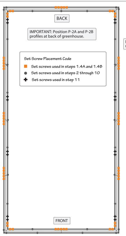
NOTE: Instructions identify sixteen set screws necessary for securing to ground in step 11.
