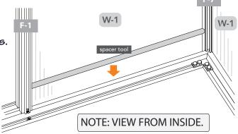
5.3D Continue working from inside left corner, place F-6 profile with mitered end next to corner and angled edge facing up onto corner W-1 panel. F-6 profile fits snugly between F-7 corner profile and F-1 wall profiles.
