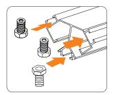
NOTE: Set screw in center bolt channel is used when installing optional shelving units. Install F-7 profile with set screw near base until needed.
