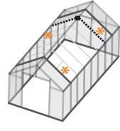
8.50 Hold two profiles together in place at ridge using one B-4 connector. Line up center hole with long hex bolt in roof ridge. Place washer on long bolt and secure all screws with three bolts.
