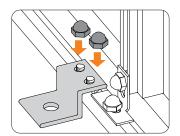
through the top of A-1 anchor to screw completely into soil. Make certain it is secured in ground.
