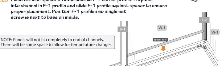
NOTE: Panels will not fit completely to end of channels.
