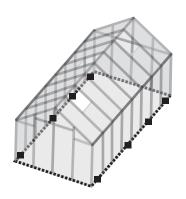
11.1 The base has predrilled holes in the inside and outside bolt channels so you can easily secure your greenhouse to a wood platform. Screw S-4 screw into hole in base
