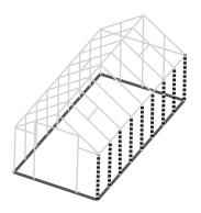
2.1A Prepare two F-7 corner profiles. Slide set screws into all three bolt tracks on one end and into two side bolt tracks on other end of corner profiles. Hand tighten each set screw to hold in place.
