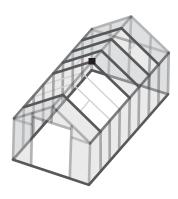
8.6D Remove plastic film from both sides of one W-1 panel. With side marked "UV Resistant" facing outside, install the next panel on the right at the back. Push panel into roof ridge channel until the other end rests on gutter ledge and then slide towards F-1 profile at back. Repeat to install W-1 panel on left.
