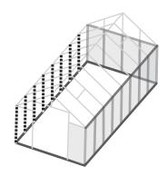
4.1A Prepare one F-7 corner profiles. Slide set screws into all three bolt tracks on one end and into two side bolt tracks on other end of corner profile. Hand tighten each set screw to hold in place.
