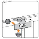
NOTE: The bottom of B-3 connector extends past the edges of side and corner profiles. B-3 connector sits on top of B-5 connector. Secure all with bolts.
