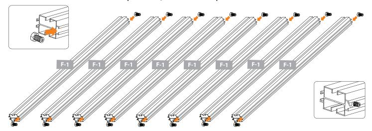
8.1B Prepare six F-1 profiles to be used with braces. Slide two set screws into bolt track on one end and one set screw on the other end of profile.
