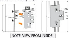
5.4F Install B-6 trim plate and secure with three bolts.
