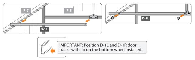
10.1C Loosen set screw in right F-7 profile and position to line up holes in D-1R as shown. Loosely secure with bolts.
