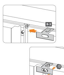
NOTE: The bottom of B-3 connector extends past the edges of side and corner profiles. B-3 connector sits over B-5 connector. Secure all with bolts.
