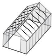
8.1A Prepare all profiles for roof. Prepare eight F-1 profiles. Slide one set screw into bolt track on each end of profile. Tighten to hold in place.
