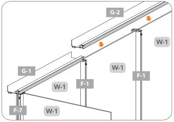
4.5B Place one set screw on the inside bolt track of the gutter at each end. Hand tighten both set screws to hold in place.
