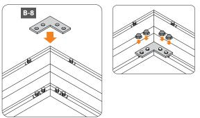
IMPORTANT: Double check the position and amount of unused set screws in the base. You should have 45 available for later assembly.
