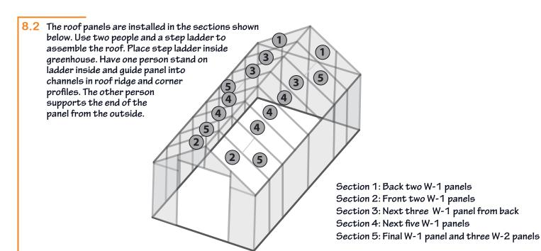
WARNING: Use two people to install roof. Allow enough time to complete this step and install and secure roof. Do not leave roof unattended until it is completely assembled.
