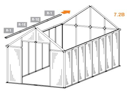
Make sure end of roof ridge is flush to profiles on front and back.
