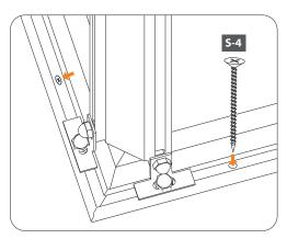
NOTE: The S-4 screw is designed to be used with wood. When securing base to foundations made of materials other than wood, use an appropriate fastener.
