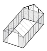
6.1A Prepare two F-7 corner profiles. Slide set screws into the same bolt track, one on each end of profile. Tighten each set screw to hold in place.
