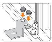
11.2B Screw each A-1 ground anchor through hole in center of bracket. Use a screw driver
