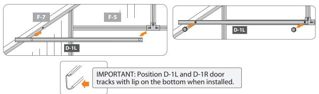
10.1C Loosen set screw in right F-7 profile and position to line up holes in D-1R as shown. Loosely secure with bolts.
