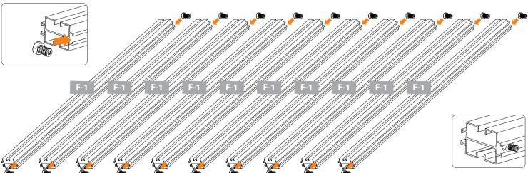
8.1B Prepare eight F-1 profiles to be used with braces. Slide two set screws into bolt track on one end and one set screw on the other end of profile.
