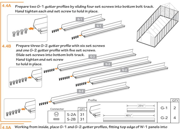
channels of gutters. Place one short G-1 gutter profile at each end and the four longer G-2 gutter profiles in the center. Seams are centered to bolt tracks in F-1 profiles.
