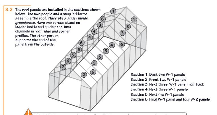
WARNING: Use two people to install roof. Allow enough time to complete this step and install and secure roof. Do not leave roof unattended until it is completely assembled.
