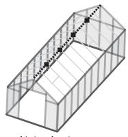
7.1 Prepare the two R-1 and three R-1E roof profiles. They will line up in a row and joined using four B-5 connectors using a total of eighteen set screws and four long hex bolts. Arrange profile so bolt track is facing up.
