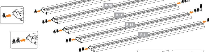
7.1B Line up five profiles in a straight line with R-1E profiles in the middle. Hand tighten set screw on each end of R-1 profile to hold in place.
