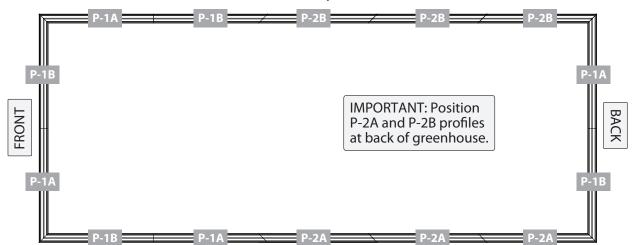
WARNING: Use extreme caution when handling profiles P-1A, P-1B, P-2A and P-2B. The bottoms may have sharp edges near the drilled holes. The cut edges on the corners of these profiles are sharp.
