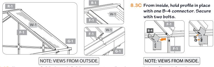
8.3D Repeat step 8.2B through 8.2C to secure install and secure F-1 profile on left side.
