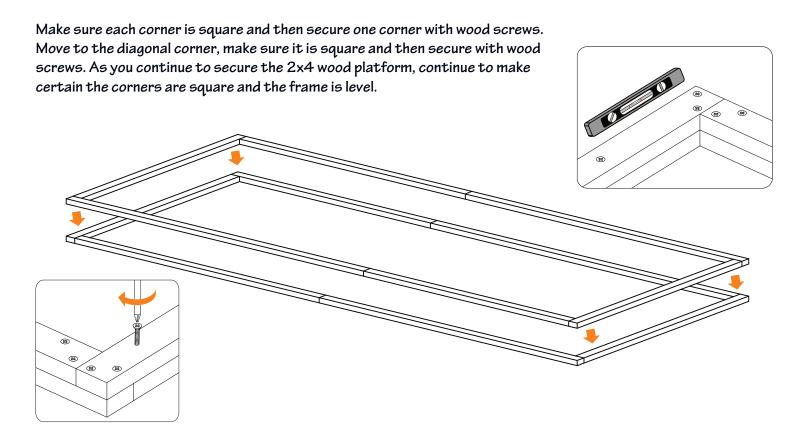
Secure wood platform every two feet with wood screws. Make certain to tighten screws into the wood platform until they are flush with the surface.
