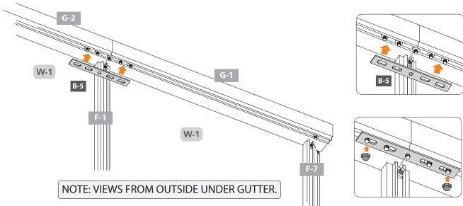
4.6C Loosen set screws on side profiles and slide down. Fit wide part of B-3 connector onto set screw, slide up into place fitting gutter set screw at other end. Tighten set screws and secure with bolts.
