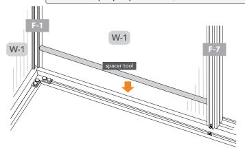
NOTE: Panels will not fit completely to end of channels. There will be some space to allow for temperature changes.
