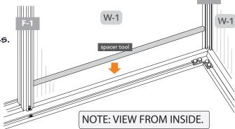
5.3D Continue working from inside left corner, place F-6 profile with mitered end next to corner and angled edge facing up onto corner W-1 panel. F-6 profile fits snugly between F-7 corner profile and F-1 wall profiles.
