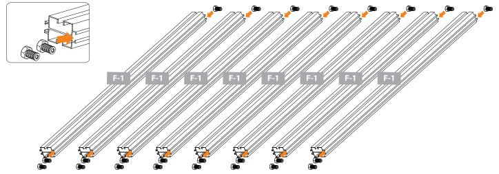
8.10 Measure 195/8 inches from one side of profile. Slide middle set screw to that point and tighten to hold in place. Tighten the other two set screws on each end of profile.
