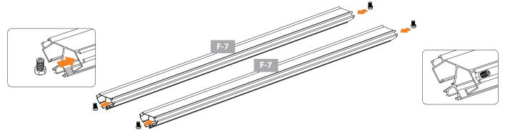
6.1B Prepare one F-2 profile. Slide set screws into both bolt tracks on each end of profile.
