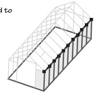
2.7B Begin at the five seams and arrange set screws so middle screw is centered. Fit B-5 connector onto gutter and hold in place using the two end bolts.
