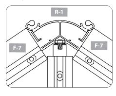
7.3A Working from inside, secure roof ridge to front end wall. Loosen set screws and adjust position to fit holes in B-7 connector. Secure with two bolts.
