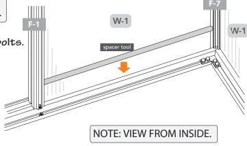
2.3D Continue building the side wall from the inside. Use the spacer with each panel and the eight remaining F-1 profiles. Repeat steps 2.3A through 2.3C.
