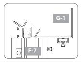
NOTE: At front and back, edge of G-1 gutter profile lines up flush with edge of F-7 corner profile.
