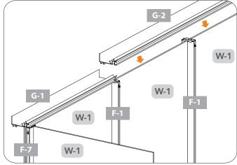
Place one set screw on the inside bolt track of the gutter 4.5B at each end. Hand tighten both set screws to hold in place.
