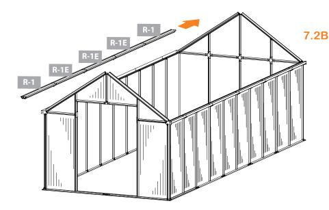
Make sure end of roof ridge is flush to profiles on front and back.
