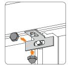
NOTE: The bottom of B-3 connector extends past the edges of side and corner profiles. B-3 connector sits over B-5 connector. Secure all with bolts.
