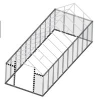
5.1 The door frame is 65¼" high from the base. To avoid adjusting the placement after assembly, prepare door frame using the exact measurements listed in these steps.
