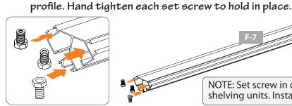
NOTE: Set screw in center bolt channel is used when installing optional shelving units. Install F-7 profile with set screw near base until needed.
