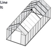
8.6D Remove plastic film from both sides of one W-1 panel.
