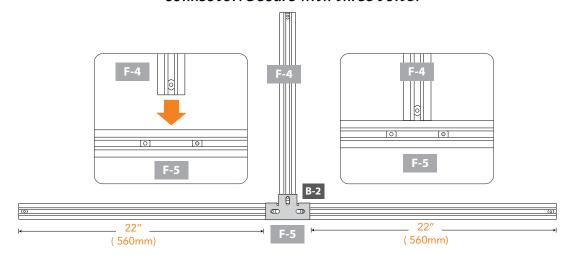
IMPORTANT: F-4 profile is centered to F-5 profile and secured on both sides with B-2 connector.
