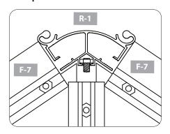
7.3A Working from inside, secure roof ridge to front end wall. Loosen set screws and adjust position to fit holes in B-7 connector. Secure with two bolts.
