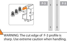
5.1B Fit B-2 connector onto profile and position so bottom of connector measures 8" from bottom of profile. Secure each with two bolts.
