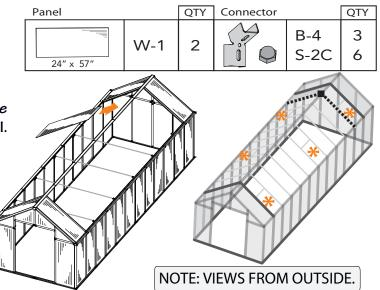
8.5C Hold two profiles together in place at ridge using one B-4 connector. Line up center hole with long hex bolt in roof ridge. Place washer on long bolt and secure all screws with three bolts.
