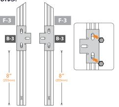
**5.2A** Prepare two F-1 wall profiles. Slide set screws into same bolt track, one on each end of profile. Position profile so set screw near base is on the inside when installed. Hand tighten each set screw to hold in place.
