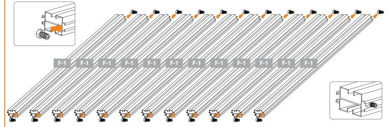
8.1B Prepare ten F-1 profiles to be used with braces. Slide two set screws into bolt track on one end and one set screw on the other end of profile.
