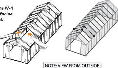
8.8F Hold two profiles together at ridge using one B-4 connector. Secure with two bolts.
