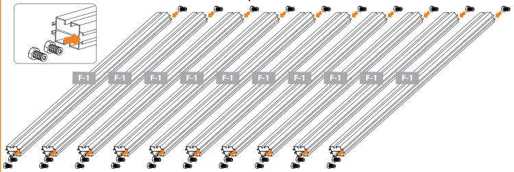
8.1C Measure 195/8 inches from one side of profile. Slide middle set screw to that point and tighten to hold in place. Tighten the other two set screws on each end of profile.
