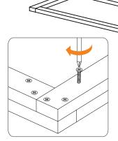
Secure wood platform every two feet with wood screws. Make certain to tighten screws into the wood platform until they are flush with the surface.
