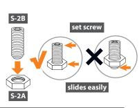
NOTE: The two pieces together is referred to in this manual as a "set screw".
