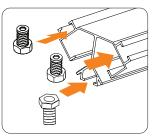
NOTE: Set screw in center bolt channel is used when installing optional shelving units. Install F-7 profile with set screw near base until needed.
