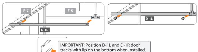
10.1C Loosen set screw in right F-7 profile and position to line up holes in D-1R as shown. Loosely secure with bolts.
