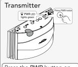
Press the **PWR** button on **transmitter** to power ON.
